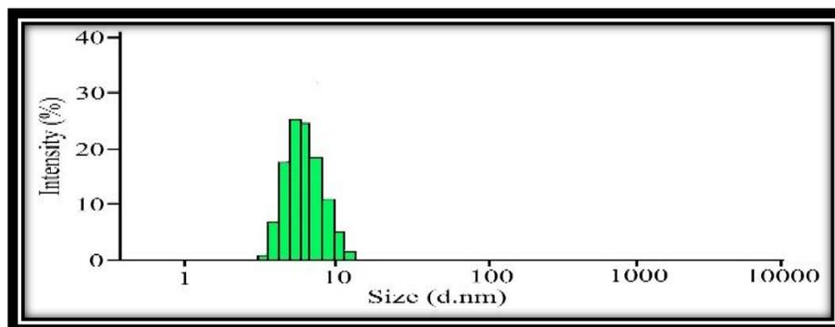
Fig. 2 (a): Size of quantum carbon dots
