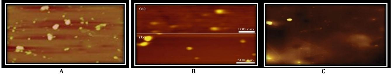
Fig. 4: Atomic Force Microscopic images (A. Chitosan; B. Carbon quantum dot; C. Nanogel)
