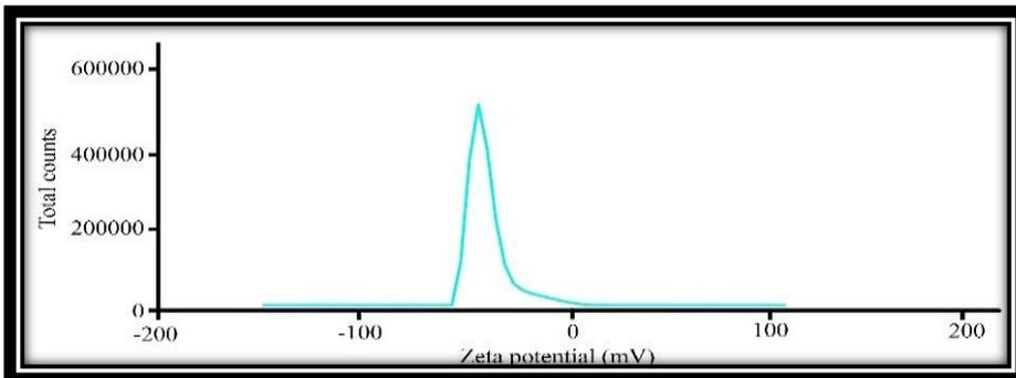
Fig. 3 (b): Carbon - Carbon Dot Zeta Potential
